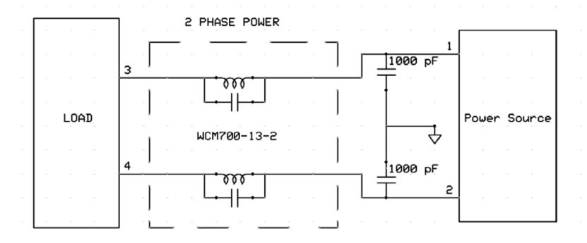
Schematic of one recommended application for WCM700-13-2
