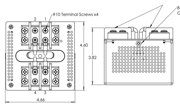
8-32 Internally Threaded Grounding Port x2
