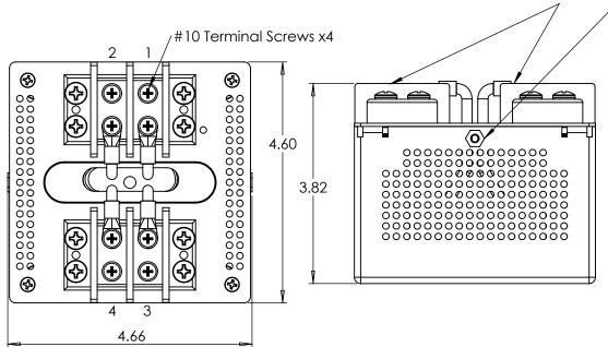
8-32 Internally Threaded Grounding Port x2
