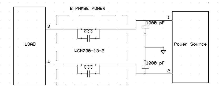
Schematic of one recommended application for WCM700-13-2
