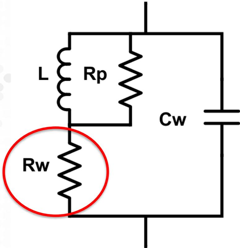
Model magnetic device per the schematic at left.
