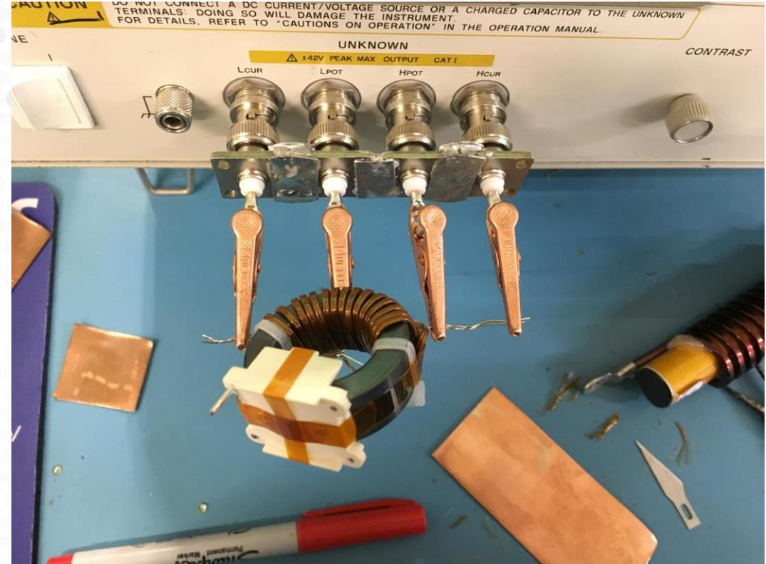
Use short fixture, with current injection and voltage measurement clips separate, to minimize stray resistance and inductance
