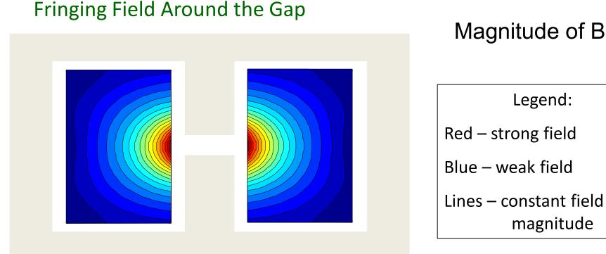
Note: the strength of the fringing field is a function of the ripple current shape and magnitude.
