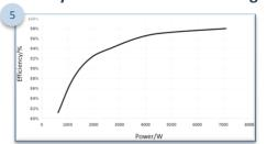
With no current oscillation(Fig 5), the designed charger successfully reached 7.2kW@98% efficiency.
