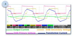
With the WCM transformer to suppress the winding capacitance, such oscillation disappeared, shown in Fig 4.
