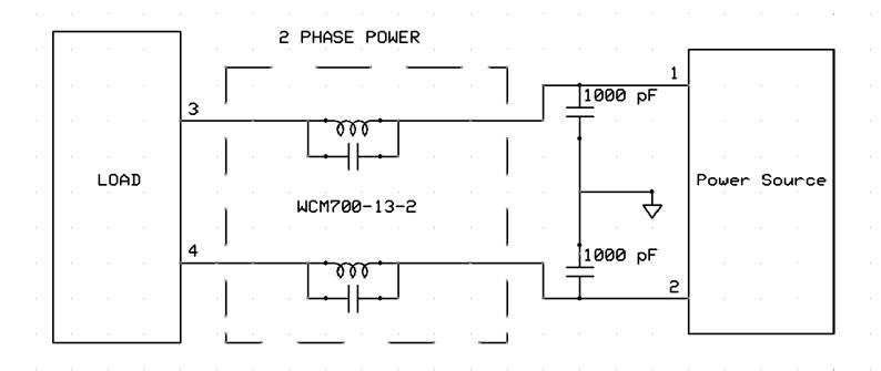
Schematic of one recommended application for WCM700-13-2
