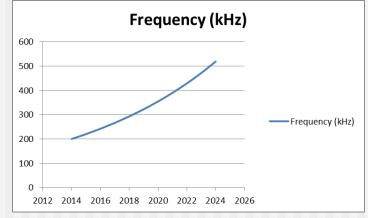
Operating frequency will increase more quickly at 10% per year. This will result in an additional 30% reduction in device volume.
