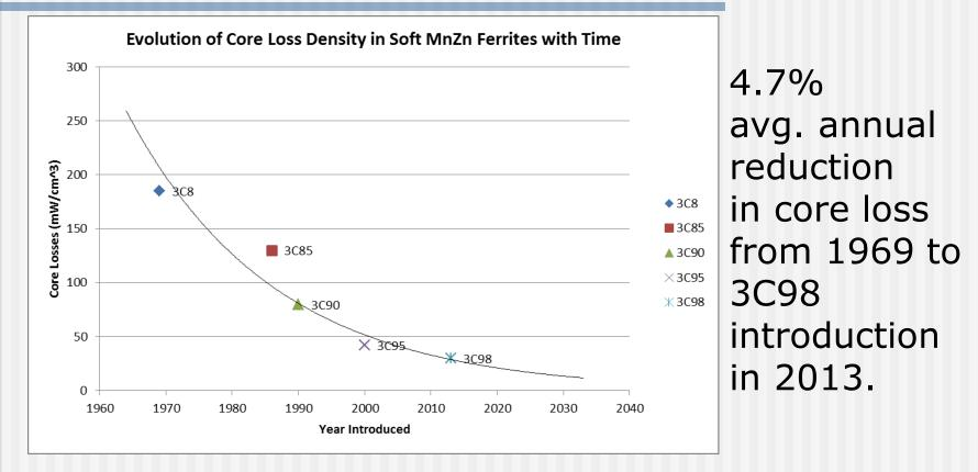
Source: Ferroxcube, Core Loss at 1 kGauss, 100 kHz
