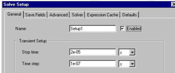
20 us (2 cycle of 100kHz) simulation time
